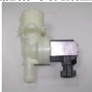
Electrovanne 6W - 2,5L/sec - 3750 \pm 10\Omega ( 20^\circ )
